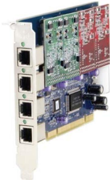
Gambar 7.1. Asterisk IP PBX Card (TDM400P)
